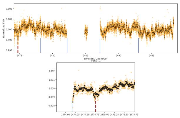
Fig 1. Full lightcurve for target TIC 248952314. The solid blue lines at the bottom of the figure indicated the times of the reaction wheel momentum dumps and the dashed black line(s) show the time(s) of the marked transit event(s). Momentum dumps occur around every 2 to 2.5 days and typically last around half an hour.
