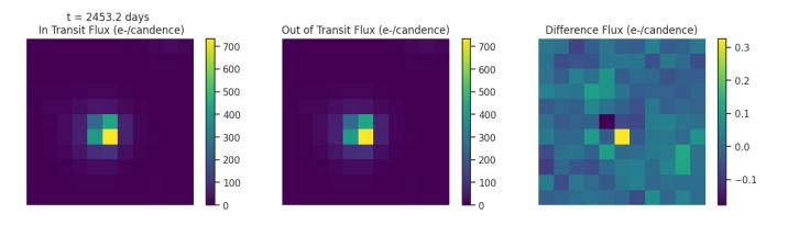
Fig 6. Difference images for target TIC 269848053 for each transit like event. Left: mean in-transit flux(left). Middle: mean out-of-transit flux. Right: difference between the mean out-of-transit and mean in-transit flux. Ensure that the change in brightness occurs on target.
